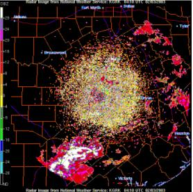
Note the extended ground clutter. The echoes to the northeast to south-south-east are all false ones. Signals were outstanding at that time.
