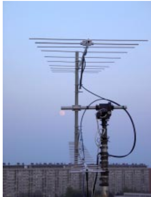
Moonrise from OK1TEH, JO70fd, Prague, Czech Republic. 100 watts on 144 Mhz. with 10 elements. QRP EME.
