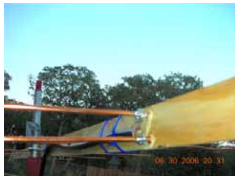
Coax is soldered directly to driven element.
